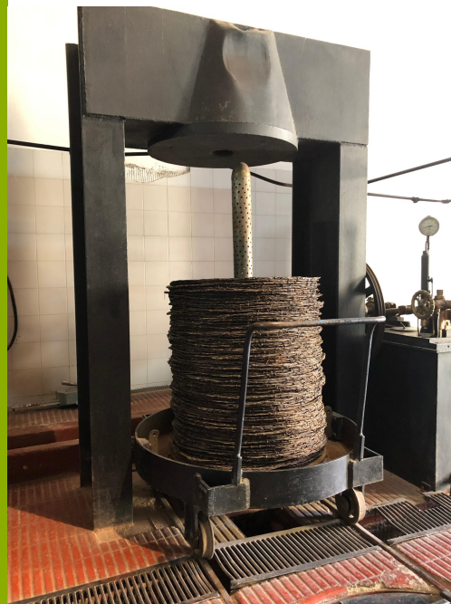
Expeller pressing olive fruits to make olive oil. Olivicula Laur - Argentina
